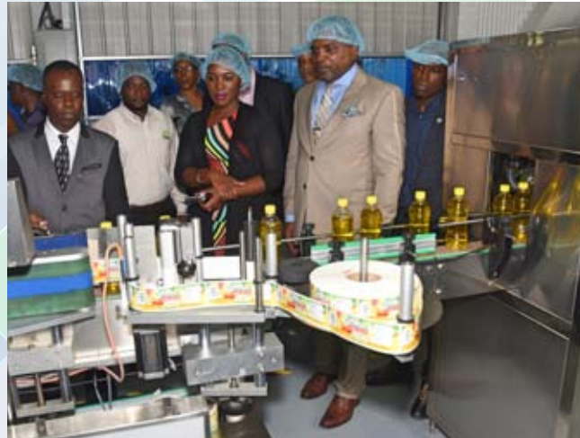
Mr. Reginald Andrews Co-Owner of Andy's Company Limited explains the various processing areas of the plant's production line to various onlookers. Shown here are the finishing processes for bottling and labelling.
